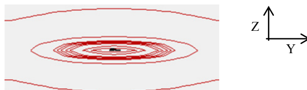
Figure 17. Electric fields in YZ view of our planar EIBT.
